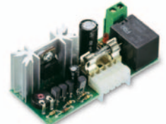
Bat K30 Plug-in card for battery charger
